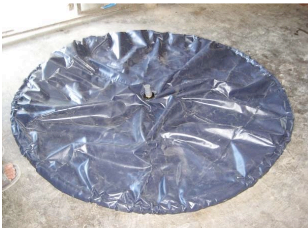
Figure 11. The HDPE top-layer with gas collection point (left) and the completed EQ1 plant with protect box and gas pipe (right)
