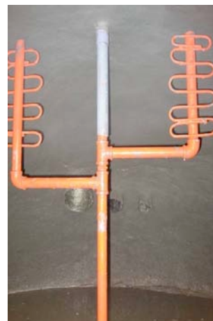
Figure 12. The completed EQ2 biogas plant with fulfilled outlet pit (left) and the crank handle installed inside digester with two blades (right) (Source: Nguyen and Do, 2009)
