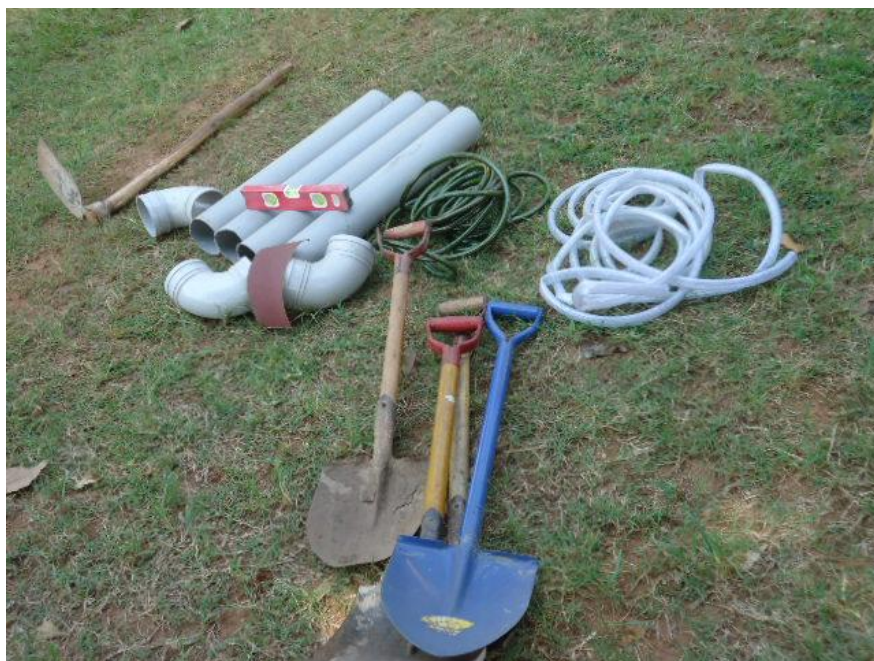
Figure 3 – Tools and materials used to install the biogas digester
