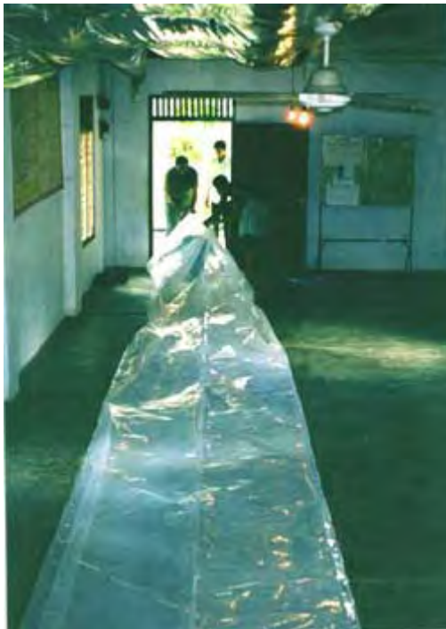
Fig. 5. Preparing the plastic bag. A person pulls one plastic bag through the other.
