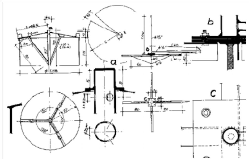
**Fig. 44:** Constructional drawing of a floating-drum plant
