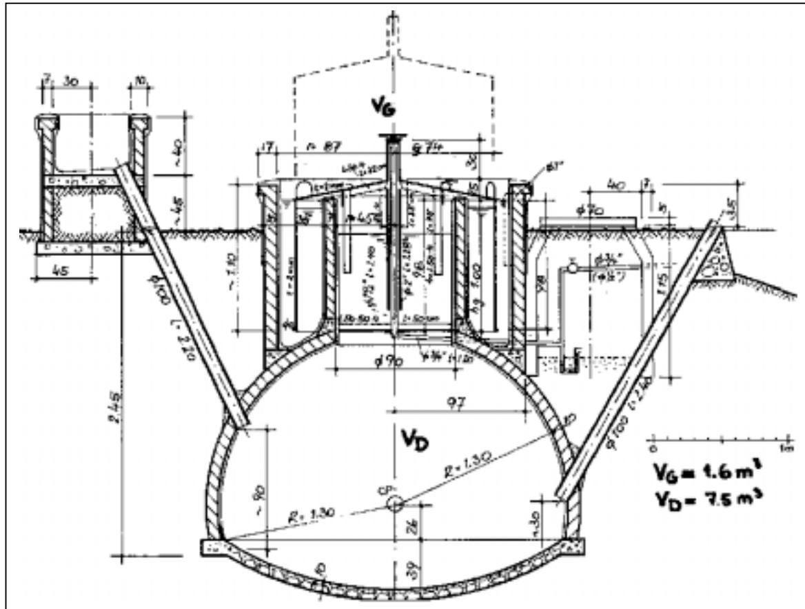
**Fig. 47:** Constructional drawing of a floating-drum plant with water jacket. Compared to the one is shown in figure 45, this plant is about 40% more expensive but can be expected to last twice as long and will handle substrate that tends to form substantial amounts of scum. Detailed building instructions for a system of this kind are available in several different languages.
