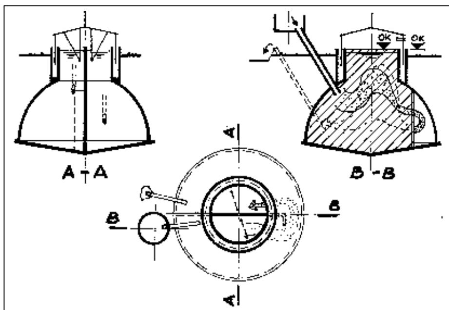
**Fig. 26:** Hemispherical plant with partition wall. The principle of the fermentation channel is obtained by the fact that the inlet and outlet pipes are close together. The partition wall extends up above the surface level of the fermentation slurry. The gasholder must therefore float in a water jacket. The "horizontal KVIC gobar gas plant", which is similar in design, works perfectly with high gas production.
