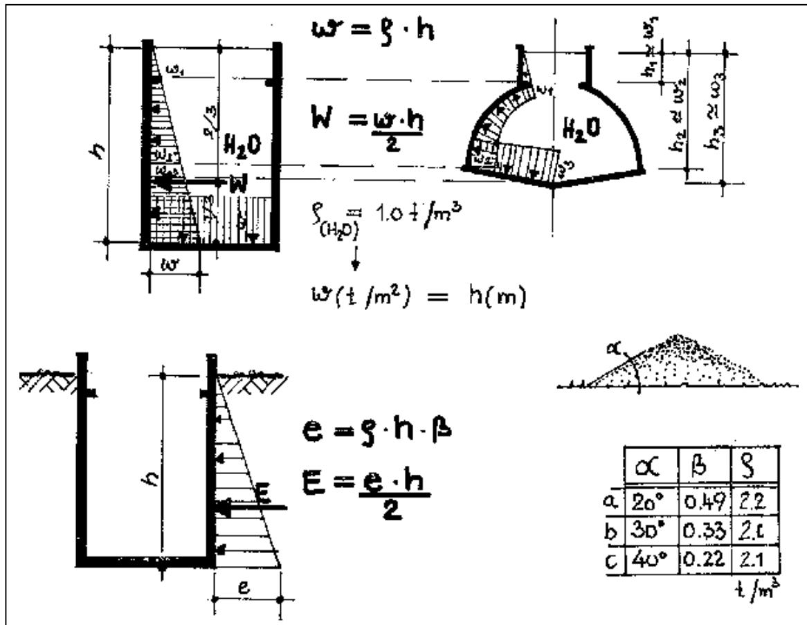
**Fig. 57:** Water pressure and earth pressure Water pressure depends directly on height. The amount of water has no effect on the pressure. The earth pressure depends on height, the angle of repose ( $\alpha$ ) and density ( $\gamma$ ) of the earth. In the table, (a) is soft loam or clayey sand, (b) is pure sand and (c) is marl or murrum.
