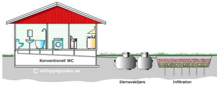
Figure 2: .A private small scale sewage plant for WC and greywater connected to a three-chambered septic tank with following infiltration. (Source: ©avloppsguiden.se)
