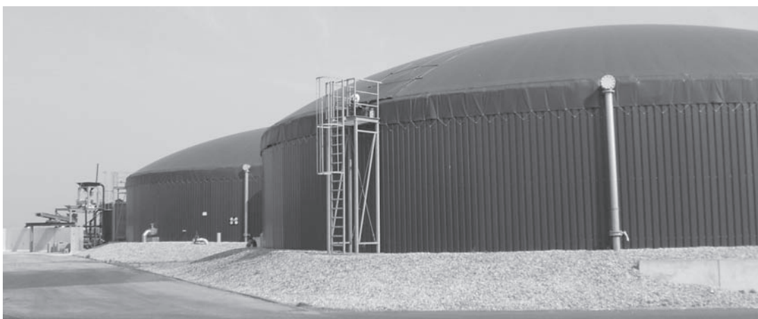
Figure 1: A 'typical' process vessel (fermentor) often used in the Netherlands. The co-fermenting takes place in a large silo covered with a flexible plastic sheet to collect the produced biogas (Heezen et al, 2010).
