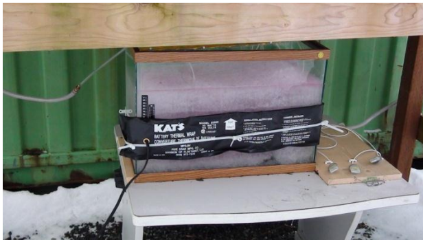
Aquarium pictured here with a car battery jacket in an effort to thaw out the tank. The jacket worked very well and was used periodically to prevent freeze up.
