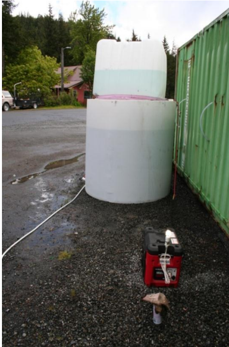
Biogas being used to power a generator. Note the additional water weight used to increase the pressure of the gas supply for running an electrical generator. The water weight was not required for cook stove operation on biogas.
