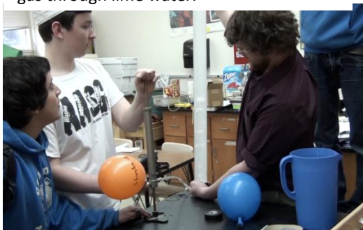
Student Keegan Crowley performs a calorimetry experiment to test the heat content of biogas prior to purifying the gas through lime water.
