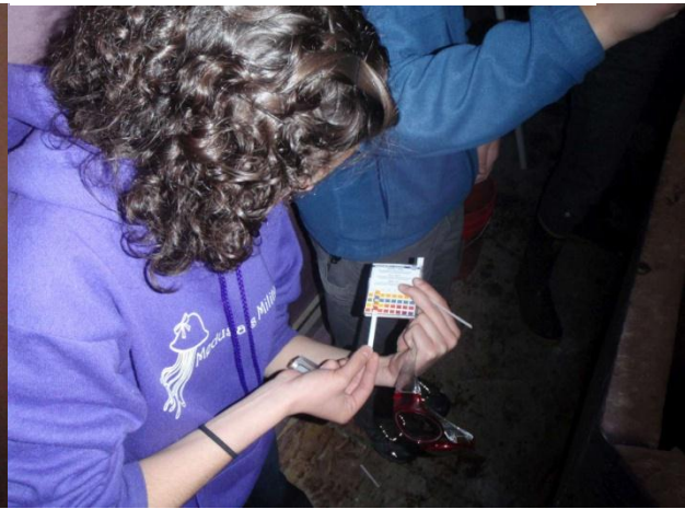
CHS student monitors chemistry by measuring pH with litmus paper. As of April 14, pH measurements are made with an Oakton PC510 meter.
