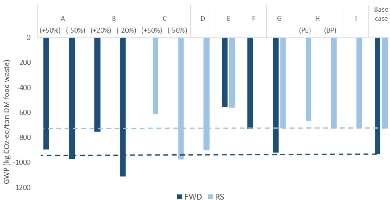
Figure 18. GWP from FWD and RS systems; base case and results from performed uncertainty and sensitivity analyses (absolute numbers). Dotted lines represent GHG-emissions from FWD and RS systems in the base case in order to facilitate comparisons.
