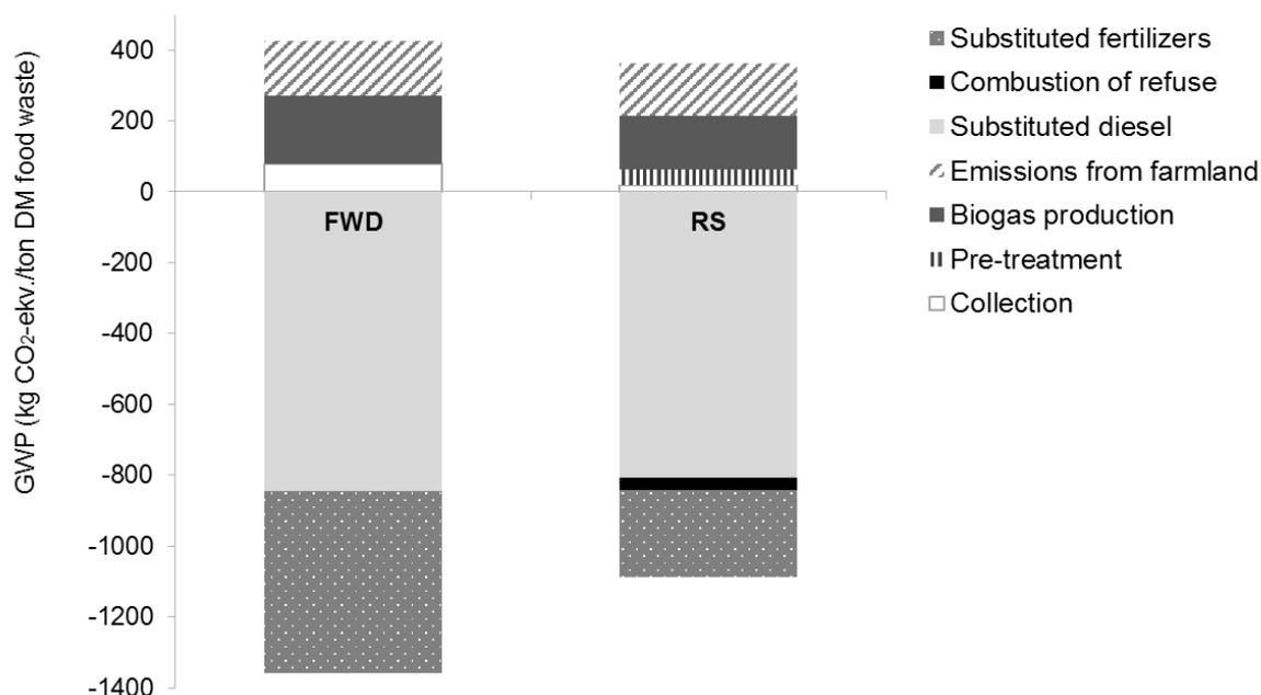
Figure 16. Overall emissions of GHG from compared systems. FWD = Food waste disposer system. RS = Reference system. The category “Collection” includes material and energy needed for disposal.
