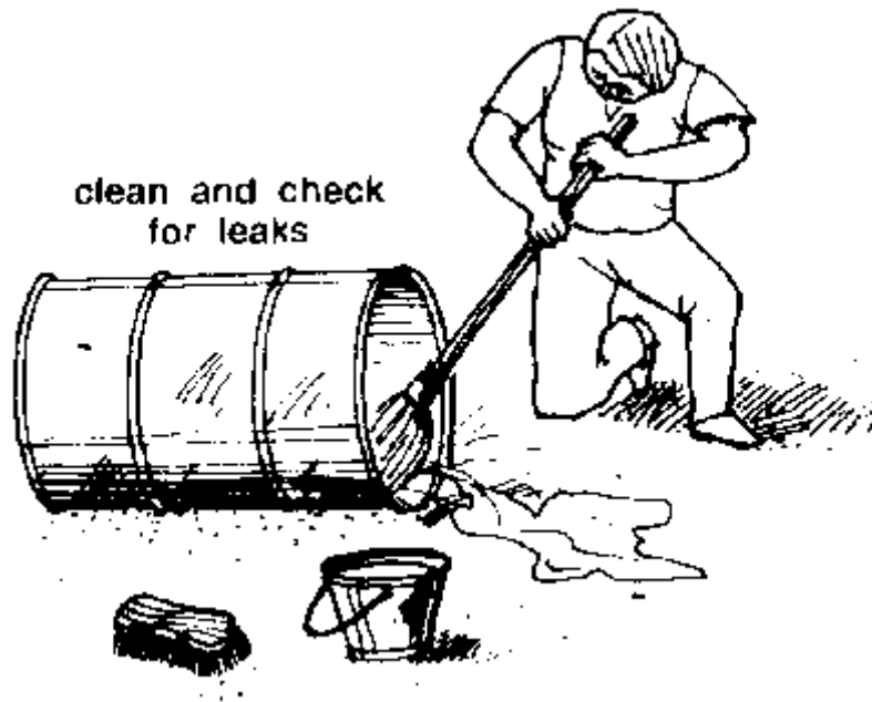
Clean and check for leaks
