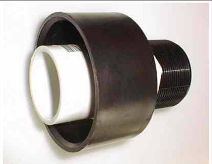
Closeup of top of HX assembly showing 2" PVC bulkhead fitting inserted into hole drilled through 4" ABS cap.
