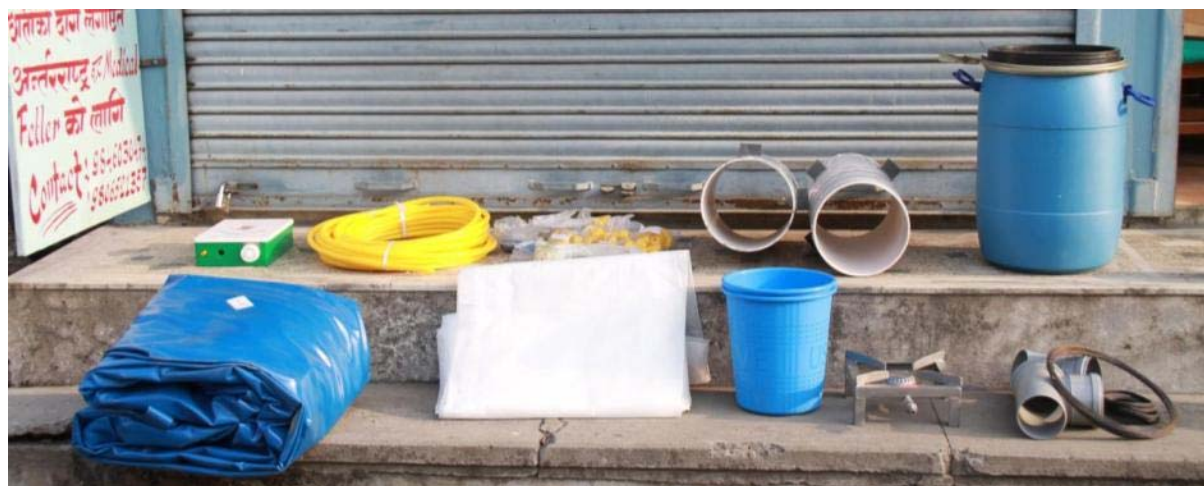
Picture 15: All materials needed for the Bag Digester in the light design.
