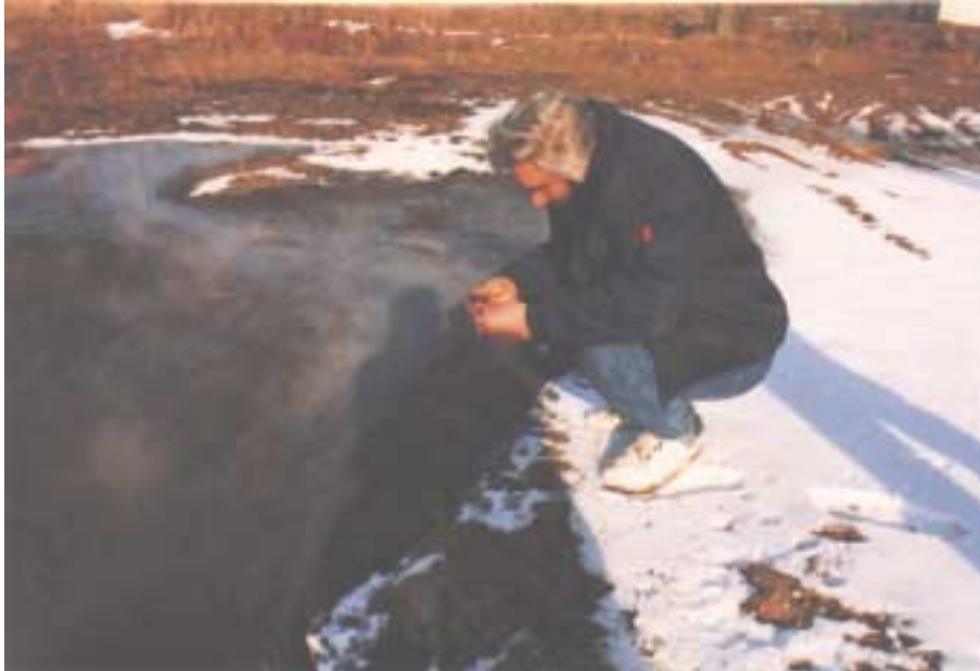
Picture 3-5 Surprising for the Lithuanians, Mr. Jensen demonstrates the necessity to literally grip the problems from their most practical side. On the picture Mr. Jensen analyses a manure sample taken from the sand outlet in the bottom of one of the digesters. There has been a periodical problem that the manure outlets of the digesters blocked. The conclusion was that the high contents of sawdust sedimented in the digester and blocked the outlet. The solution was more frequently emptying of the sand outlet and more operation with the agitators when fresh manure was added, and digested manure should escape through the manure outlets. This should avoid sawdust blocking the outlet, and help to transport sediments out of the digester.
