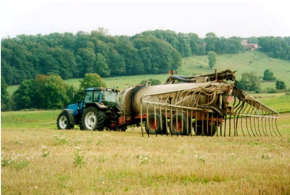
Figure 4.2.1 Hose spreader for spreading liquid manure, Helsingborg
