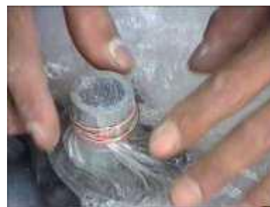
Photo 26. Covering the gas outlet with a plastic bag
