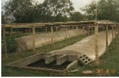
Photo 97. The use of plastic biodigesters to recycle the manure from a unit with 100 sows (1000 pigs in total) in Pozo Verde farm, Jamundi, Colombia
