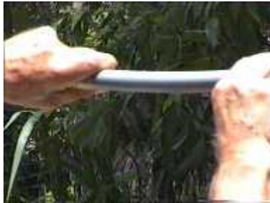
Photo 79. Make a hole in the PVC pipe, take the water out and stick it again with tape or a rubber band (# 6-2)
