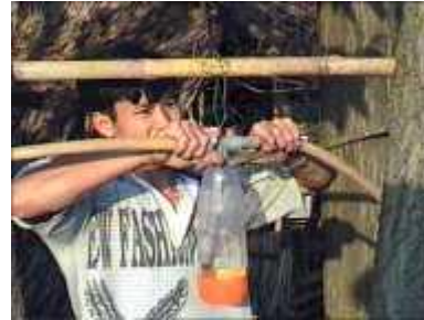
Photo 50. Joining the other end of the PVC "T" to the plastic hose that goes to the reservoir bag
