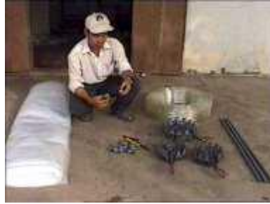
Photo 11. Materials for installing a plastic biogas digester
