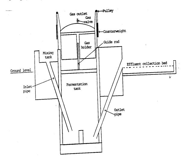
Figure 2. A Typical Indian Biogas Plant
