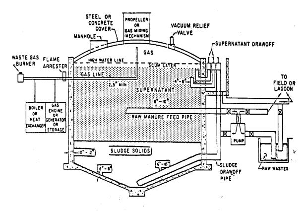
Figure 4. A Typical Fixed Wall Sewage Treatment Plant
