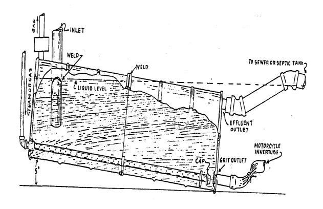
Figure 5. A Low-Technology Hybrid Digester
