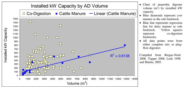
Figure 19 Installed kW by volume; EU and US data (EC Oregon, 2009)
