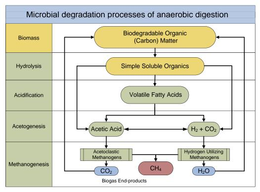
Figure 10 Microbial degradation processes of anaerobic digestion (EC Oregon, 2009)
