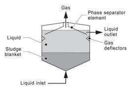
Figure 11 Upflow anaerobic sludge blanket (Scott, 2005)
