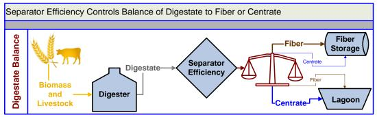
Figure 20 Separator efficiency and digestate balance (EC Oregon, 2009)
