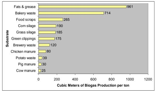
Figure 14 Cubic meters of biogas production per ton of substrate (Redrawn from Kramer, 2008)
