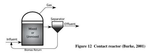
After digestion, effluent is degassed and settled in a separator or gravity tank; solids are returned to the main digester for further degradation. Mechanical methods such as centrifuges, presses, and membranes have been used to speed the separation process.
