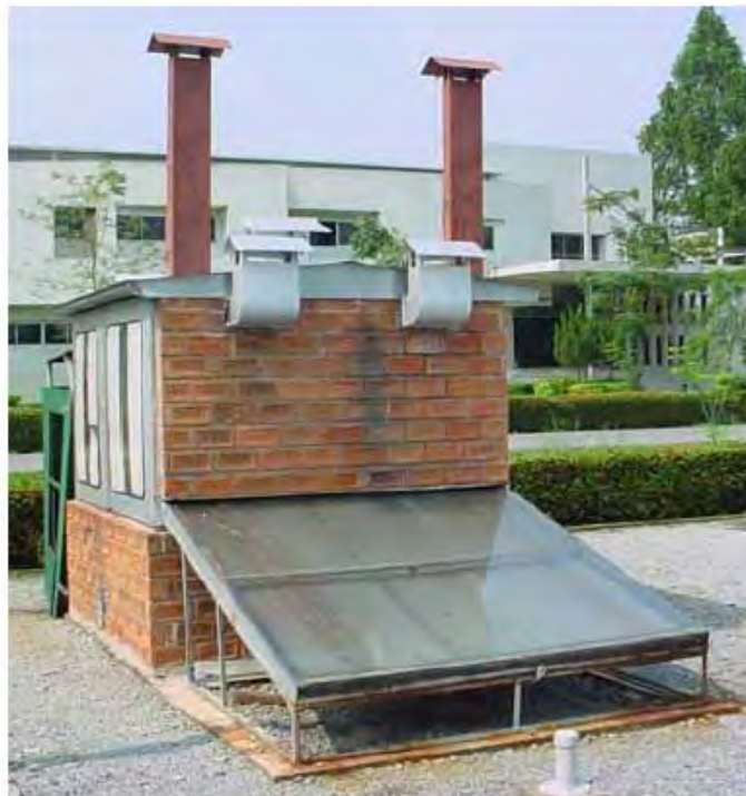
Figure 2.20: The solar-biomass hybrid cabinet dryer
