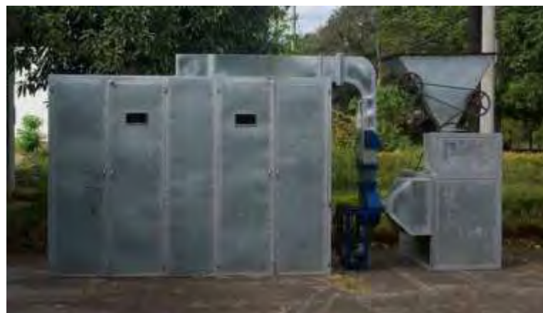
The rice husk-fuelled cabinet dryer FD-200
