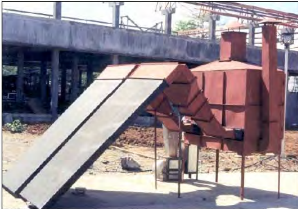
Figure 10.4: The transpired collector solar-biomass hybrid cabinet dryer
