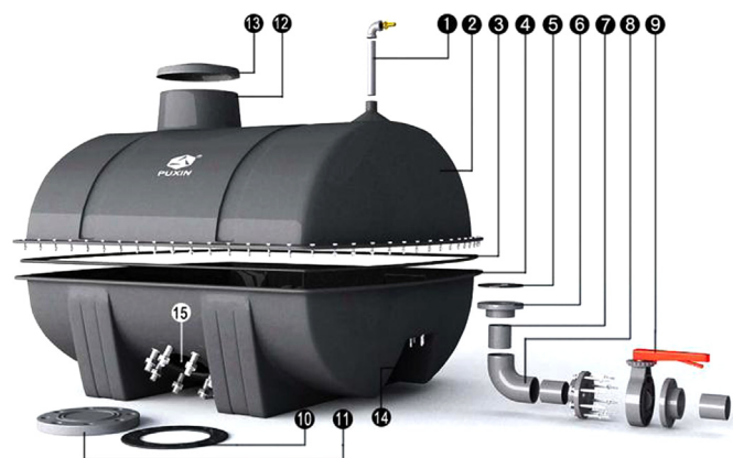
Fig. 13. Typical portable and assembled digester in Malaysia (1—Gas pipe; 2—Upper part; 3—Seal; 4—Bottom part; 5— \phi 110 Seal ring; 6—Flange; 7—Connecting pipe; 8—90° elbow; 9—Butterfly gate; 10—blind plate; 11— \phi 200 Seal ring; 12—Inlet; 13 - Cover; 14—Outlet; 15—Slag outlet), photo courtesy: Shikun Cheng.
