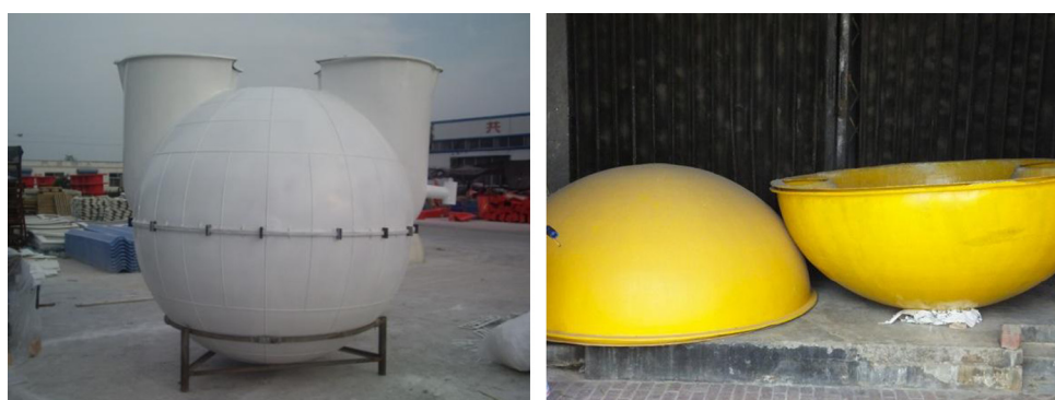
Fig. 1. (Left) A complete PBD in China and (right) top-half PBDs in Bangladesh, photo courtesy: Shikun Cheng.
