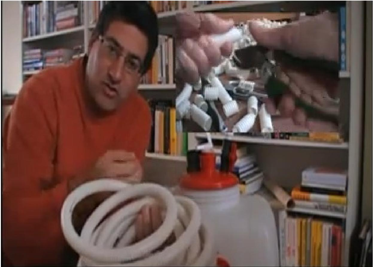
Figure 18. At an average sale price of 10 cents per plastic "bioball", the "aquarium filter" solution is too expensive for developing country applications so we have had to find ways to replicate the idea using cheaper materials, such as the corrugated plastic electrical conduit shown above. We are still uncertain as to whether the extra labor involved in chopping the conduit into bits achieves significantly better results or if we can resort to simply stacking coils of conduit in the tank.
