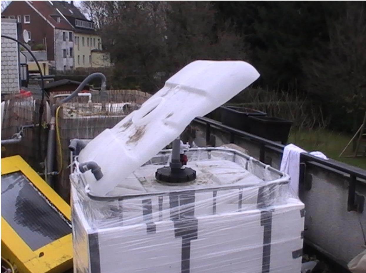
**Figure 24.** The Culhane's second family size biodigester is made from a 700 liter IBC tank nested inside a 1000 liter IBC that is insulated with styrofoam. Hot water discharged from baths and showers surrounds the internal tank and keeps the bacteria at their desired temperature.
