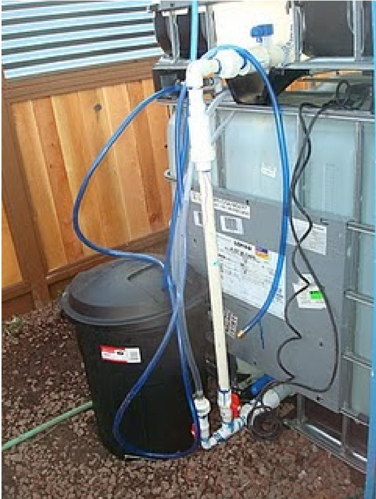
Figure 30. The plumbing set up for the Solar CITIES gas collection system
