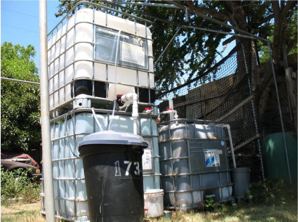
Figure 28. Figure showing how gas is piped from digester to collector
