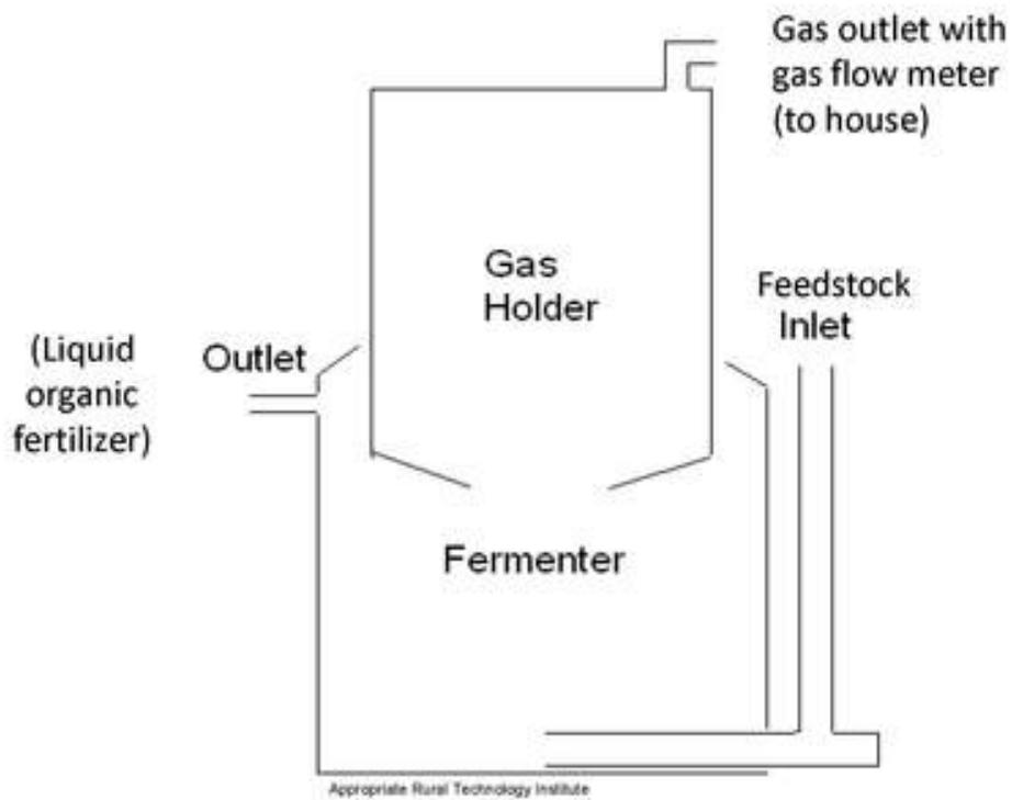
Figure 1. This is the simplest of possible biogas systems that can be constructed, and can be done so using two water tanks or even plastic trash cans.
