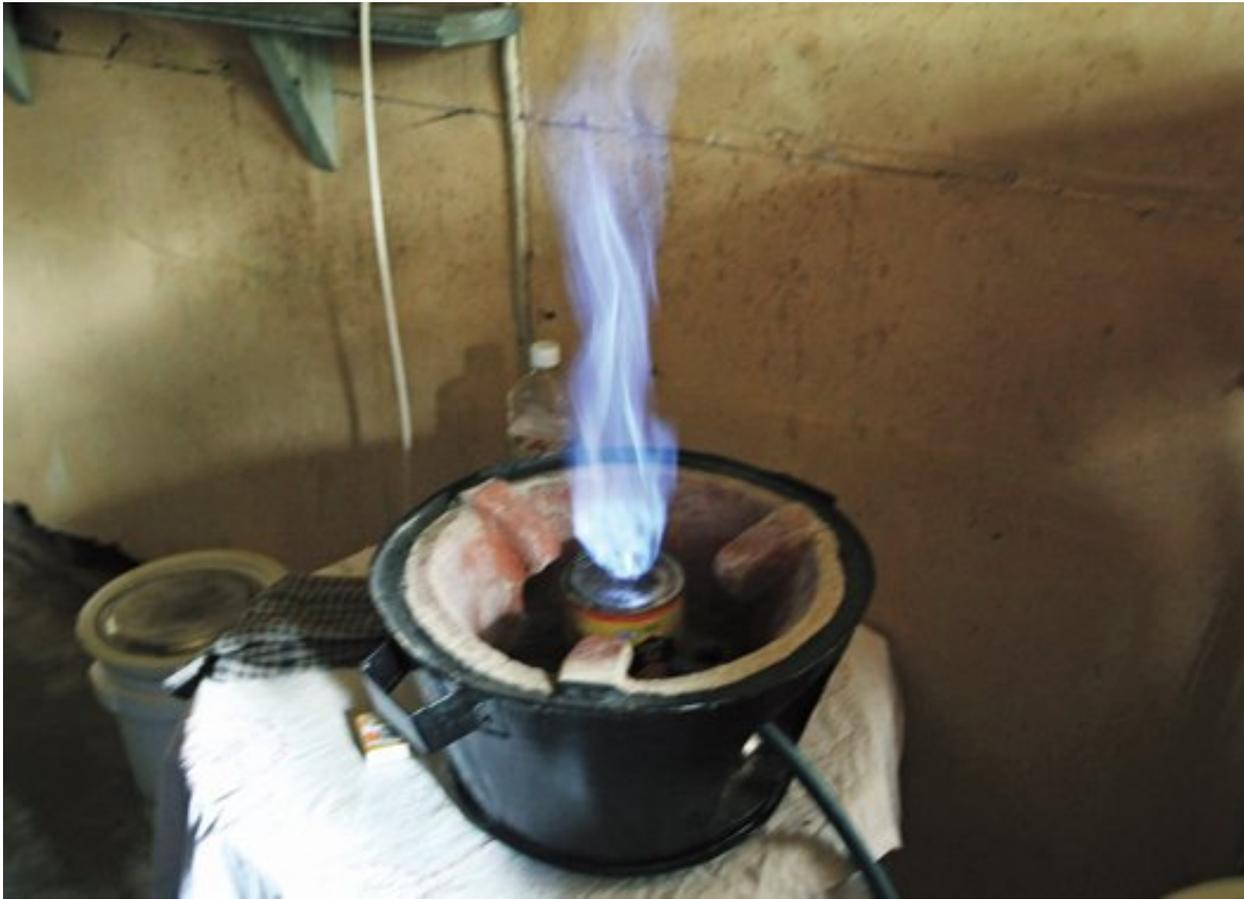
Figure 6. At the Jamhuri Energy Centre, which develops local alternative-energy systems, Elizabeth N. Kimonge and Dominic Kahumbu Wanjihia build hybrid clay stoves optimized for biogas that can also use traditional wood or biochar fuels. The biogas is piped into a removable coffee can filled with stones with a perforated lid. When the gas runs out the coffee container can be simply removed and biomass put in to continue cooking.
