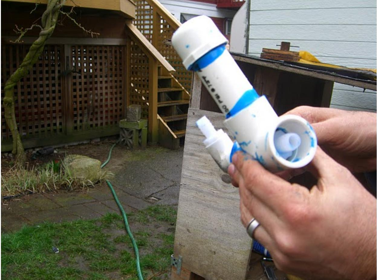
Figure 32. The heat exchanger plumbing
