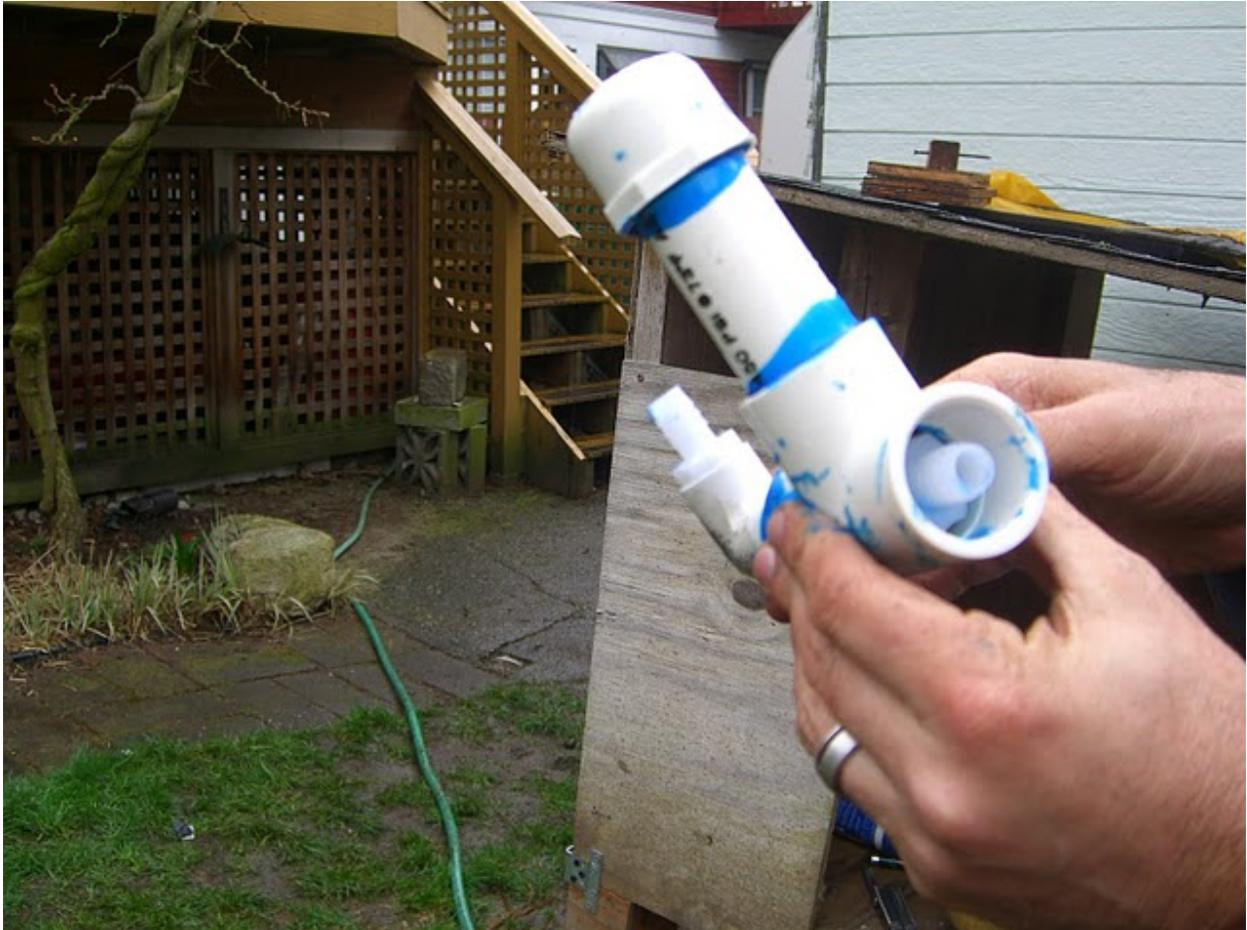
Figure 32. The heat exchanger plumbing
