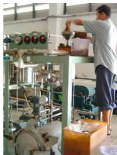
Fig. 8.5.4. Prototype of steam explosion unit.
