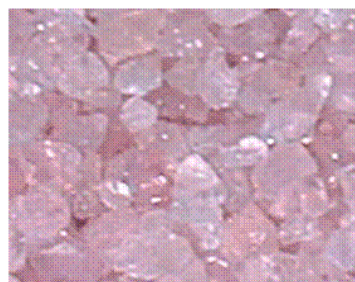
b) Silica gel turns pink once it has soaked up moisture.
