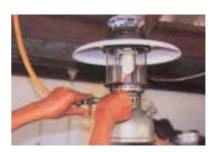
☐ When the brightness is low and the gauze mantle is flaming, adjust the nozzle to the left with tongs or up and down until the light is bright again.
