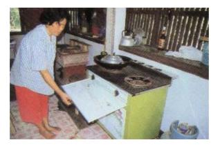
☐ For a stove with built-in cooking vessel built into the stove, remove the tray under the stove to clean.
