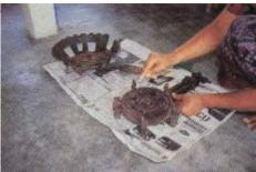
☐ Always clean the burner by removing the head burner and pushing through the holes with a sharp wooden stick, wire or nail so that gas will flow out easily. Use a wire brush to get rid of sediment. Later scrub the rust or dirtiness out.
