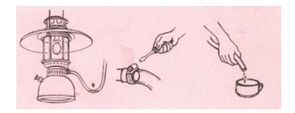
☐ Rubber hose should be checked every month for any water. Valve should be closed and hose emptied if there is water trapped inside. Hose clamp must be tightened after replacing the hose.
