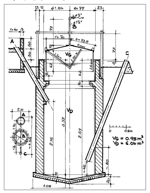
Fig 50: Constructional drawing of a floating-drum plant for quarrystone masonry (vertical plant)
