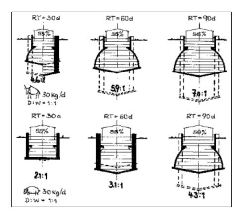
**Fig. 12:** Dependence of shape on retention time on a floating-drum plant (cattle dung above; pig manure below) Filling volume and gasholder capacity (C = 55 %) are the same in each case. The differences in digester/ gasholder ratios result solely from the differing retention times (RT).
