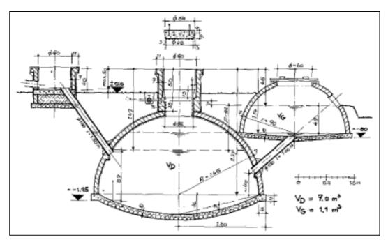
Fig. 49: Constructional drawing of a fixed-dome plant with upper opening
