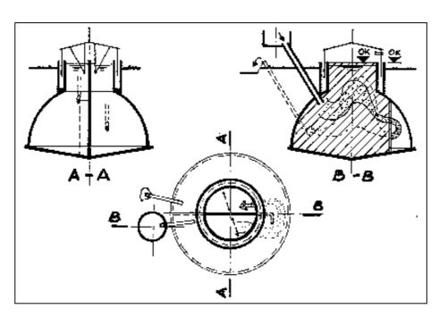
**Fig. 26:** Hemispherical plant with partition wall The principle of the fermentation channel is obtained by the fact that the inlet and outlet pipes are close together. The partition wall extends up above the surface level of the fermentation slurry. The gasholder must therefore float in a water jacket. The "horizontal KVIC gobar gas plant", which is similar in design, works perfectly with high gas production.
