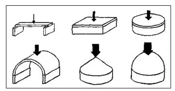
Fig. 16: Shape and load-bearing capacity.
