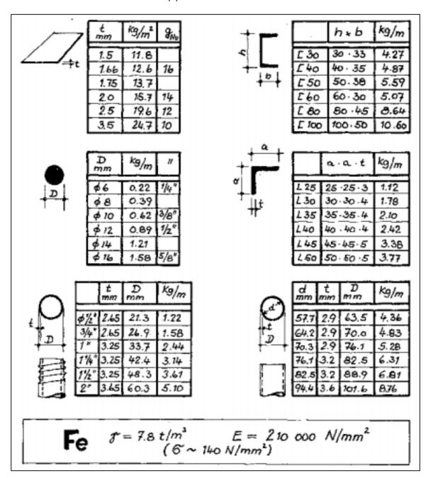
Fig. 59: Cross sections of common steels and pipes
