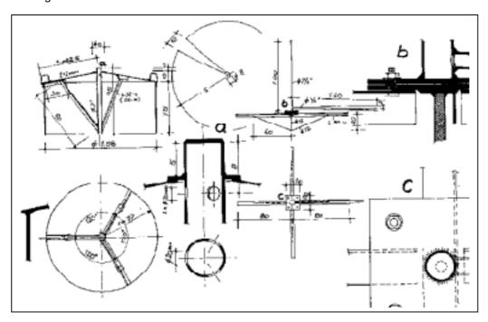
Fig. 44: Constructional drawing of a floating-drum plant
