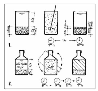
Fig. 22: T esting of mortar sand 1. Fines (loam, dust): Water glass 1/3 sand. 2/3 water, stir vigorously. Leave to stand for one hour. Measure fines. A maximum of 10 % of the amount of sand is permissible. 2. Organic matter: Bottle with stopper (not cork) to be filled with 1/3 sand and 2/3 soda lye (3 %). Shake repeatedly within an hour. Leave to stand for 24 hours. Water colour clear or light yellow: good; red or brown: bad.
