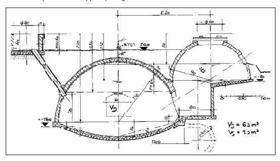
Fig. 48: Constructional drawing of a fixed-dome plant without upper opening
