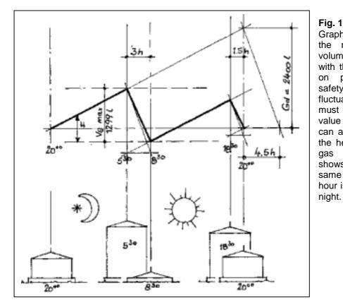
Fig. 10: Graphic determi-nation of the required gasholder volume in accordance with the second example on page 23/24. The safety margin of 25 % for fluctuating gas production must be added to the value VG. The distance H can also be regarded as the height of the floating gas drum. Experience shows that about the same volume of gas per hour is produced day and
