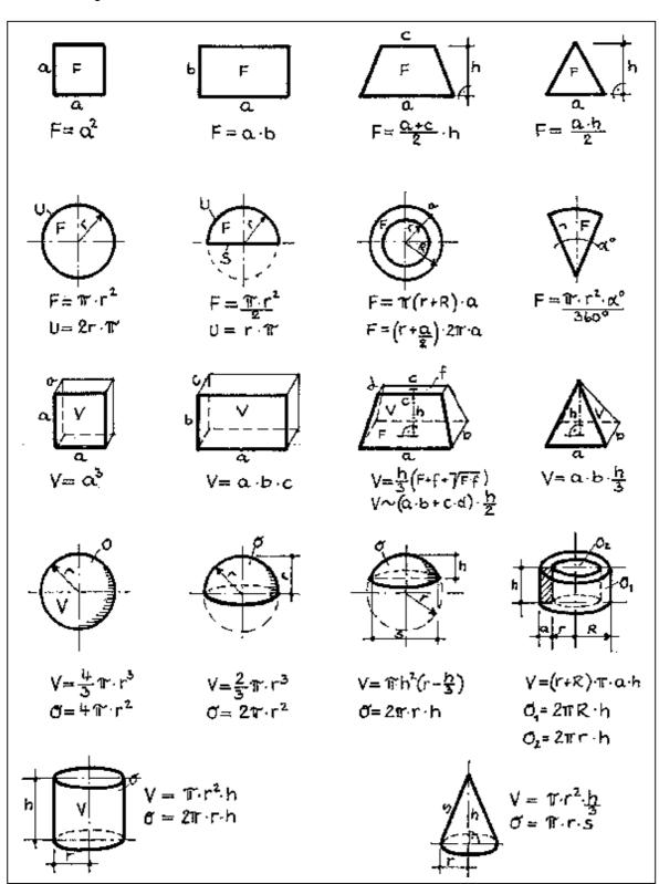
Fig. 55: Fundamental geometric formulae
