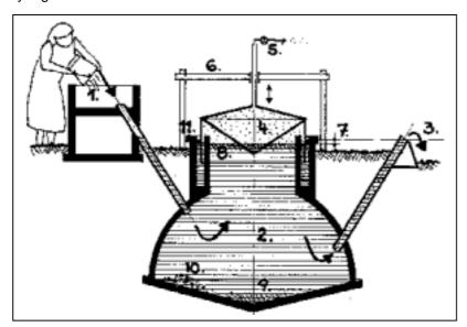
**Fig. 5:** Floating-drum plant 1. Mixing tank with inlet pipe. 2. Digester. 3. Overflow on outlet pipe. 4. Gasholder with braces for breaking up surface scum. 5. Gas outlet with main cock. 6. Gas drum guide structure. 7. Difference in level = gas pressure in cm WC. 8. Floating scum in the case of fibrous feed material. 9. Accumulation of thick sludge. 10. Accumulation of grit and stones. 11. Water jacket with oil film.
