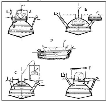
Fig. 3: plants Simple biogas Floating-drum plant B Fixed-dome plant C Fixed-dome plant with separate gasholder. The pressure is kept constant by the floating gasholder. The unit can be operated as a continuous overflowtype plant with no compensating tank. The use of an agitator is recommended. D Balloon plant E Channel-type digester with folia and sunshade
