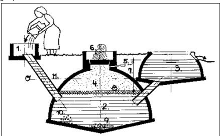
**Fig. 4:** Fixed-dome plant 1. Mixing tank with inlet pipe. 2. Digester. 3. Compensating and removal tank. 4. Gasholder. 5. Gaspipe. 6. Entry hatch, with gaslight seal and weighted. 7. Difference in level = gas pressure in cm WC. 8. Supernatant scum; broken up by varying level. 9. Accumulation of thick sludge. 10. Accumulation of grit and stones. 11. Zero line: filling height without gas pressure.
