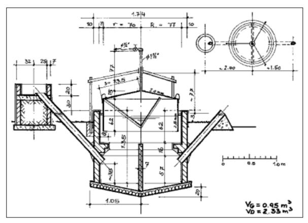
Fig. 51: Constructional drawing of a plant with an extremely low digester/gasholder volume ratio
