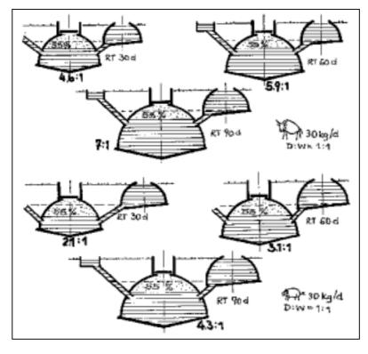
Fig. 13: Dependence of shape on retention time on a fixed-dome plant (cattle dung above; pig manure below) The filling volume and gasholder capacity (C = 55 %) are the same in each case. The differences in digester/ compensating ratios tank result solely from the different retention time (Gd as a result of RT, Figures 7 and 8).
