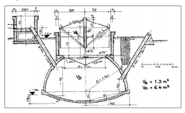
Fig. 45: Constructional drawing of a floating-drum plant with an internal gas outlet and no water jacket
