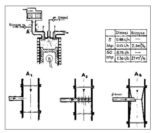
Fig. 42: Gas connection to diesel engine.
