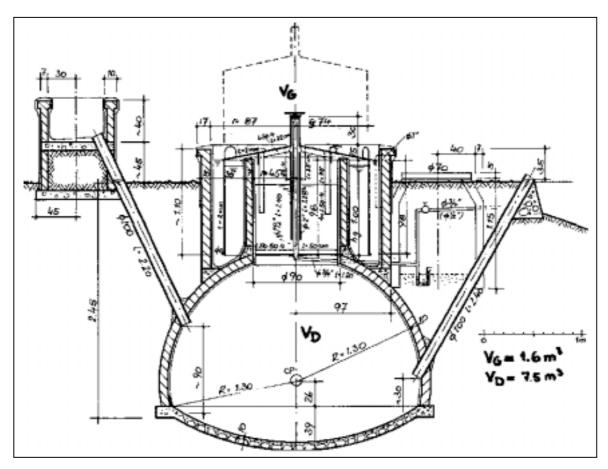
**Fig. 47:** Constructional drawing of a floating-drum plant with water jacket. Compared to the one is shown in figure 45, this plant is about 40% more expensive but can be expected to last twice as long and will handle substrate that tends to form substantial amounts of scum. Detailed building instructions for a system of this kind are available in several different languages.
