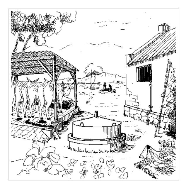
Fig. 1: A farmyard biogas plant
