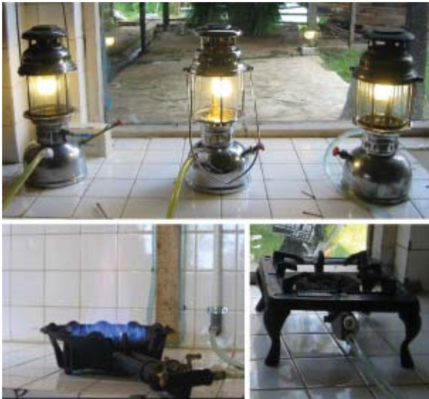
Figure 5. Utilization of biogas for mantle lamp and gas stove.
