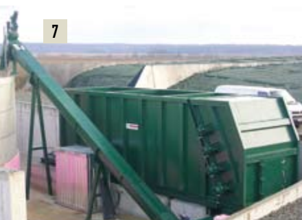
Photo 7: Silage dosing unit (back) with spiral elevator (front). The silage clamps can be seen in the back.
