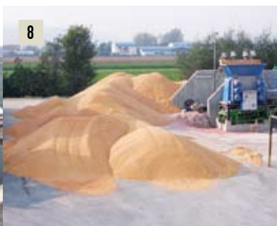
Photo 7: Silage dosing unit (back) with spiral elevator (front). The silage clamps can be seen in the back.
