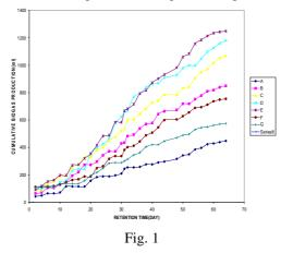
The graphs show a progressive increase in the cumulative biogas production for digester A to G. This could be attributed to the fact that anaerobic digestion of organics proceed best if the fermentation slurry consists roughly of about 8% total solid content [7]. The gradual decrease observed in F and G could be ascribed to the fact that the total solid content in both digesters are beyond the specified range for optimal biogas production.
