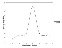
Fig 2 Plot of Average Rate of Biogas Production versus Saw dust Concentration
