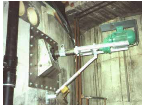
Figure 19: Stirring device for a european biodigester
