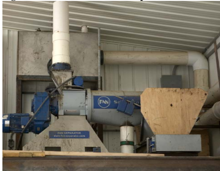
Figure 40 – Screw Press Solids Separator
