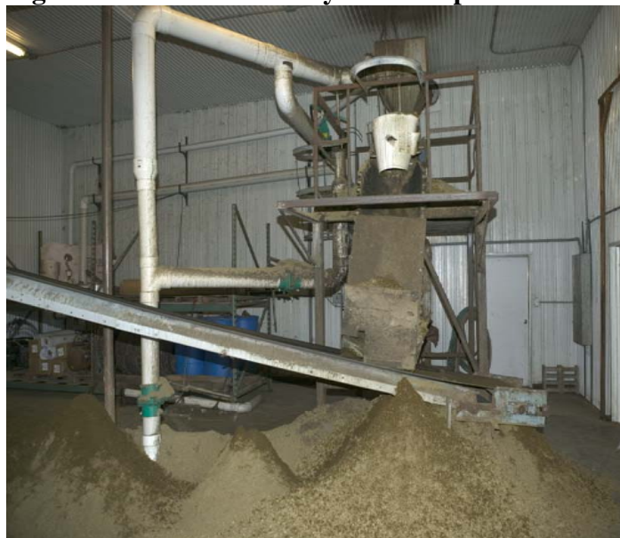
Figure 18 – Double S Dairy Solids Separator
