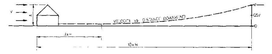
Fig. 3.3. Wind velocity (V) pattern between barns. The effect of one building on the next was estimated by using the empirical formulas for wind breaks. The effect of the shape of the barn was examined using empirical formulations for gravity up-tlow ventilation in chimneys.
