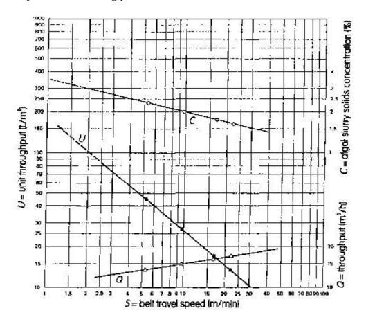
Fig. 7.4. Operational performance curves of the filter belt algae harvester: Q = USB/60; U = 182S-0.844 (from data shown); and B is the belt width (0.95 m for Singapore machine; 12- $\mu$ m polyester belt fabric).
