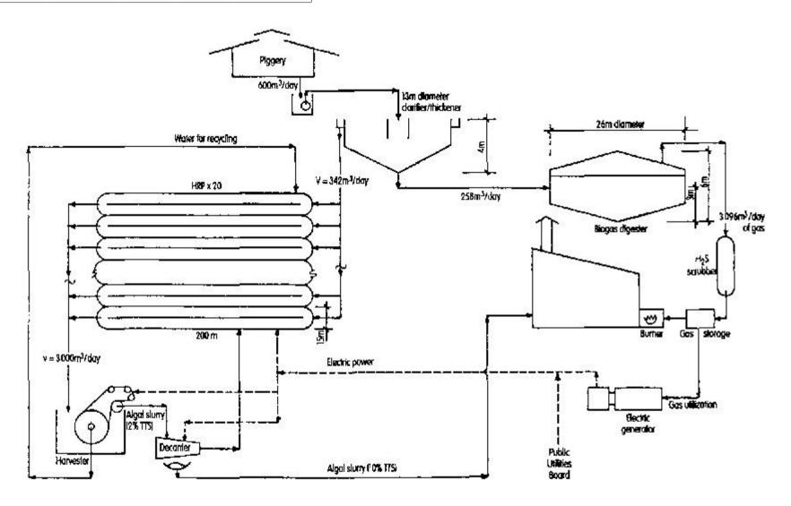
Fig. 7.7. Layout of high-rate algae pond (HRP) system used in the economic feasibility analysis (30 000 SPP).
