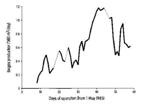
Fig. 10.8. Biogas production of the PPP digester.
