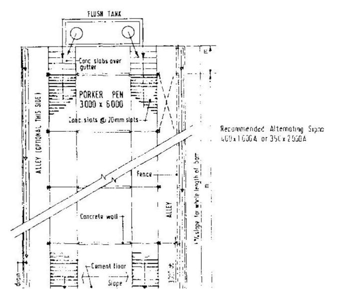
Fig. 4.6. Weaner to porker barn (all dimensions are in millimetres except as indicated). This concept was first implemented on the industrial farm, where five barns were built in 1982 and 1983. Each barn was 282 m long and contained 1 800 porkers.
