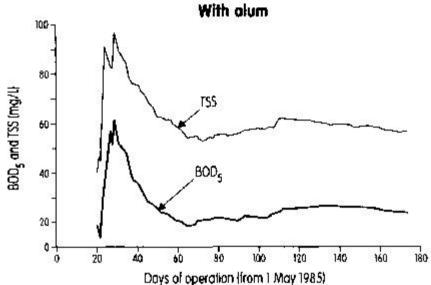
Fig. 10.5. Running means for BOD5 and TSS of clarifier effluent.
