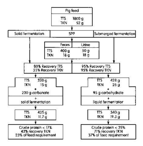
Fig. 8.1. Flow of TTS and nitrogen in fungal fermentation.
