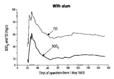
Fig. 10.5. Running means for BOD5 and TSS of clarifier effluent.
