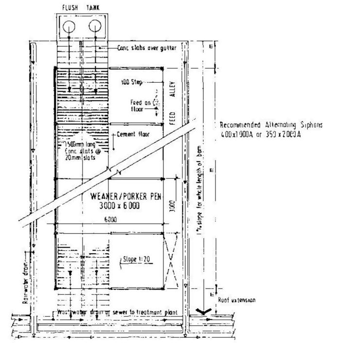
Fig. 4.5. Weaner-grower-porker barn with sloped floor (all dimensions are in millimetres, except as indicated). Grower pens should have 0.5 m² of floor space per pig. For good performance, and to discourage such problems as tail biting, no more than 25 pigs should be put in one pen.
