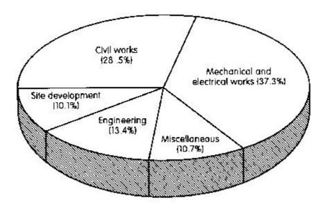
Fig. 9.5. Five major cost components of PPP construction.
