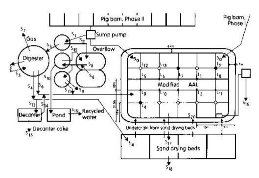
Fig. 10.4. Points of composite sampling of the aerated anaerobic lagoon
