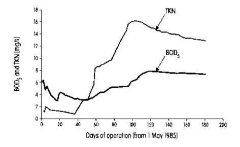
Fig. 10.6. BOD5 and nitrogen content (TKN) of recycled water.
