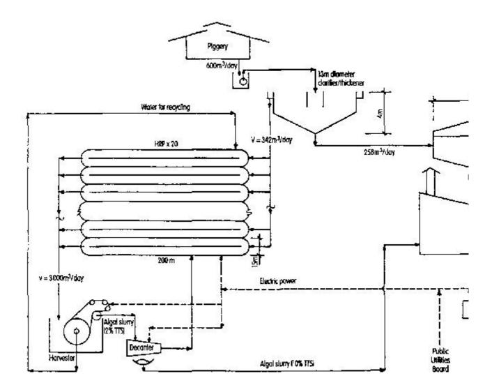
Fig. 7.7. Layout of high-rate algae pond (HRP) system used in the economic feasibility analysis (30 000 SPP).
