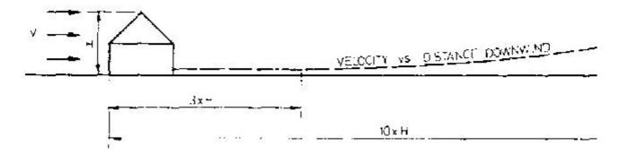
Fig. 3.3. Wind velocity (V) pattern between barns. The effect of one building on the next was
