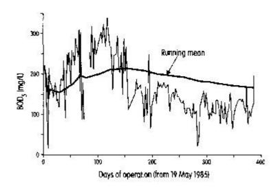
Fig. 10.3. BOD5 moving average of PPP lagoon effluent.
