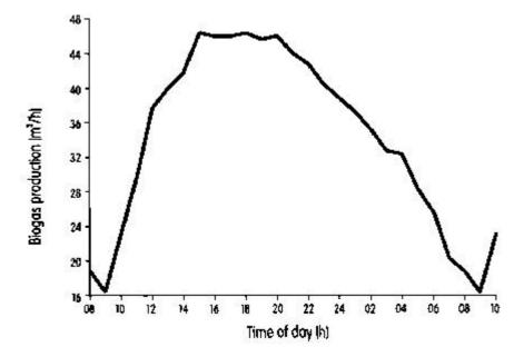
Fig. 10.9. Hourly rate of biogas generation by the PPP digester.
