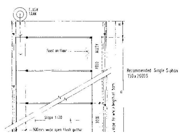
Fig. 4.7. Open-gutter flushing porker barn (all dimensions are in millimetres, except as indicated). This system was tried in the experimental barns at PPRTI. During hot weather, the pigs tended to lie in the gutter and impede the flow of the flushing water.
