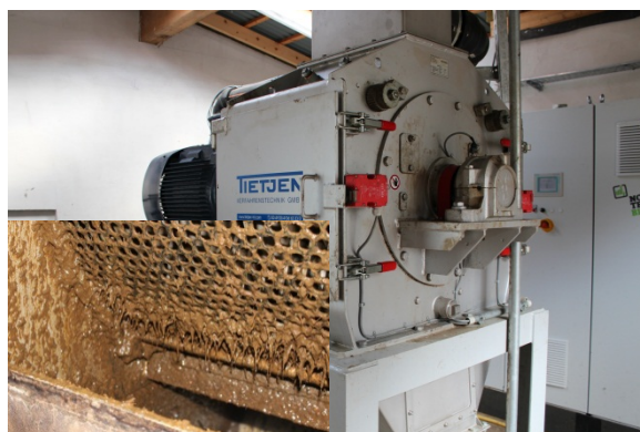
Figure 22: For medium sized and large biogas plants, disintegration techniques like this combination of hammer mill and specific microorganisms, can improve efficiency and reliability. Photo: F. Gerlach, FiBL.
