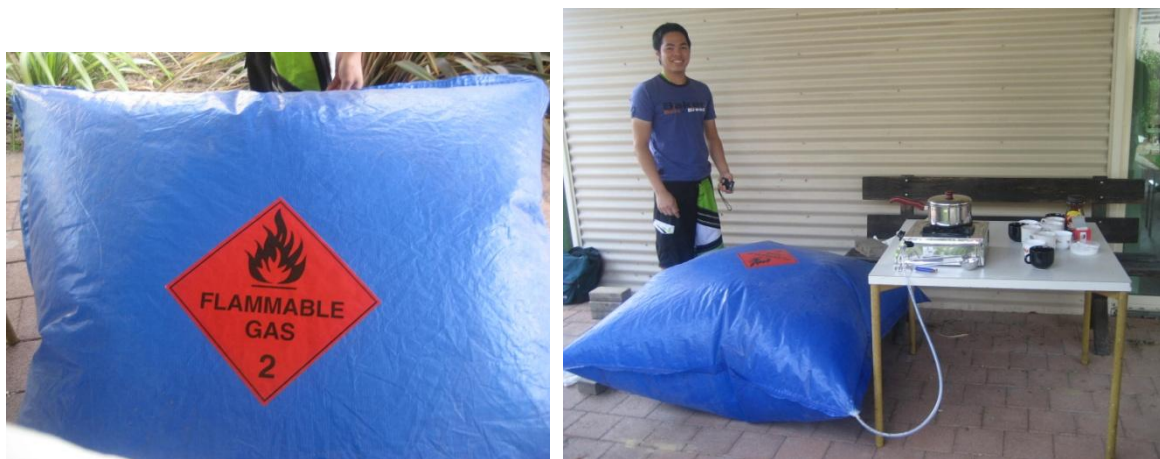
Fig 2. Biogas collected and used for cooking from the treatment of food waste
