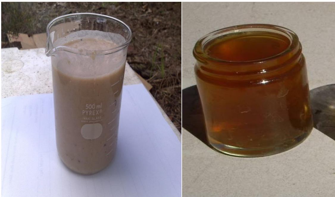
Fig 3. Pulped meat and bakery waste (left) and the treated digestate from the digester
