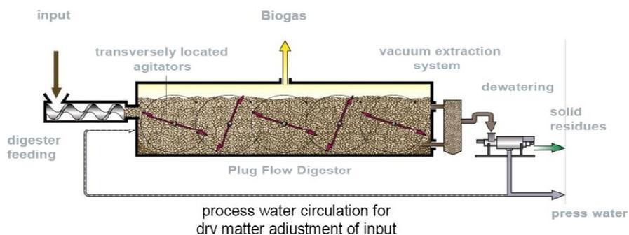
Figure 1: Principle of the LARAN<sup>®</sup> recumbent plug-flow dry digester
