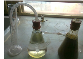
Figure 6: Risen slurry in the digester
