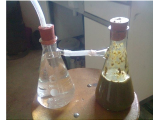
Figure 4: Unrisen slurry in the digester
