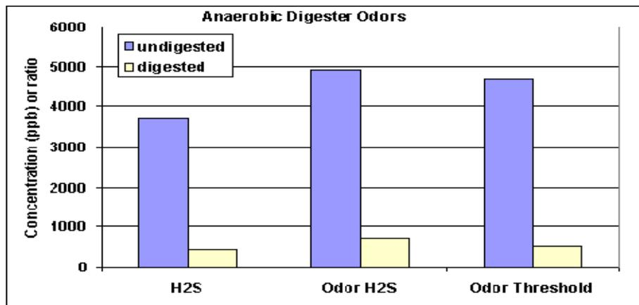
**Figure1** Hydrogen sulfide and odor threshold in gases from digested and undigested manure [Loimor, 2000].
