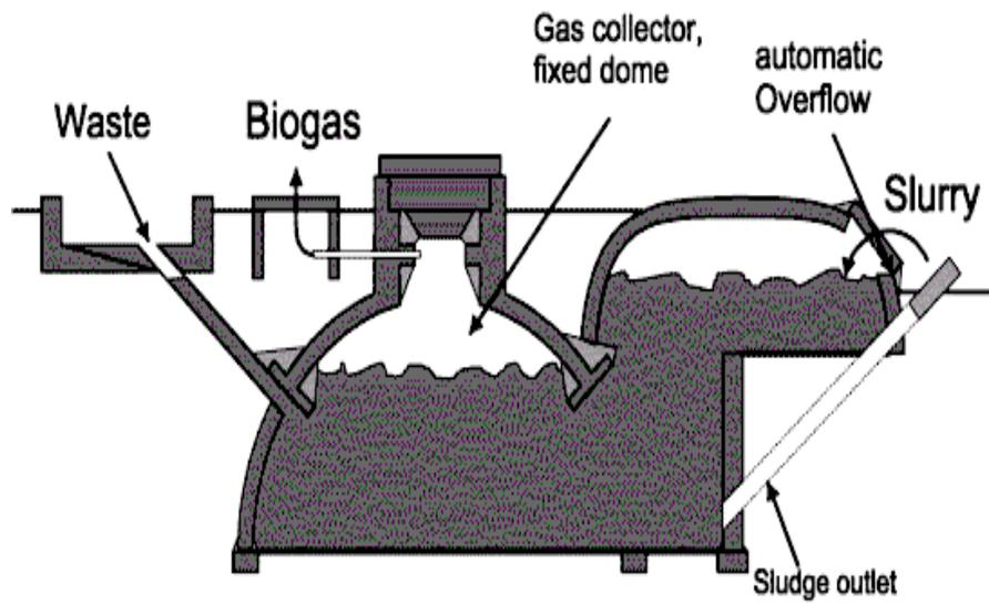
Figure 6 Fixed dome plant CAMARTEC design
