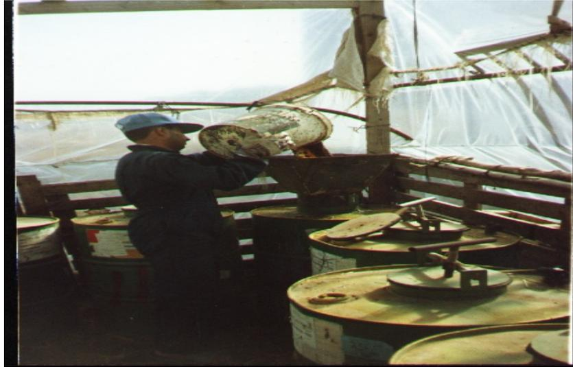
**Photo 6** Introducing sample into the digester
