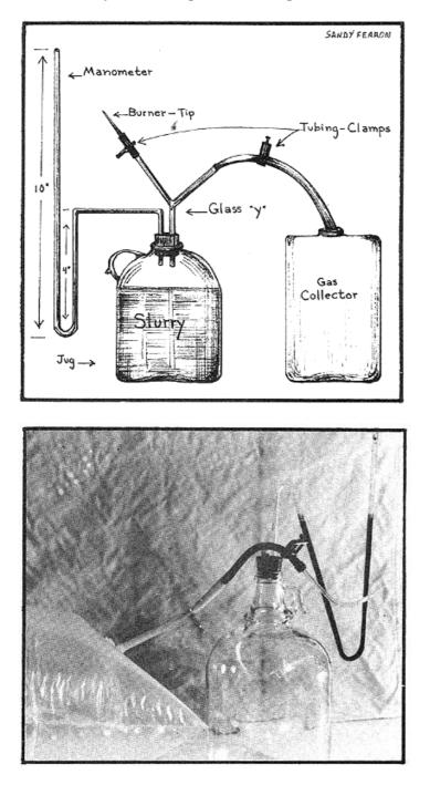
Start your generator working with all its valves (clamps) closed and, after a couple of days, the water being "pushed" up the long arm of the manometer will indicate that
