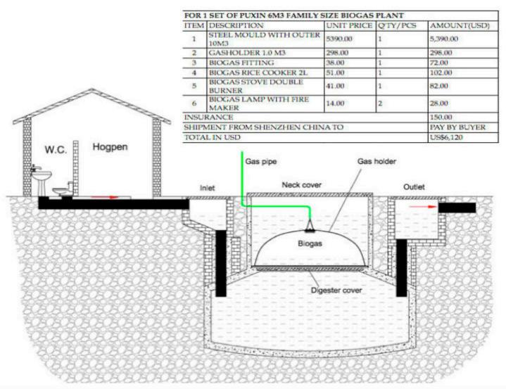
With 10 m3 family size Puxin biogas plant as per the above drawing, enough biogas can be provided to 2 families of 4 persons each for cooking and lighting. By making use of steel mould with outer 10 m3 to construct, which is can be reusable for many times.
