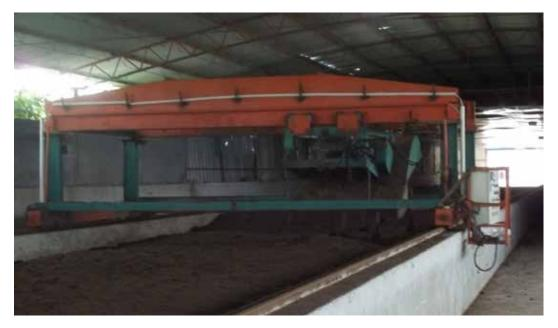
Automated compost making system which processes digestate for application back to fields and sale.
