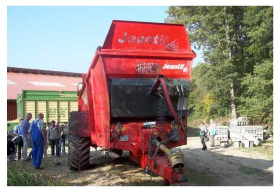
Spreader used for putting digestate onto the fields.
