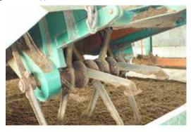
Aeration types on the compost making system for turning compost.
