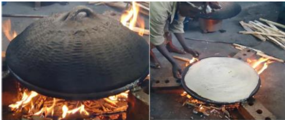
Figure 1. 2 Traditional 3 stone biomass injera baking stove
