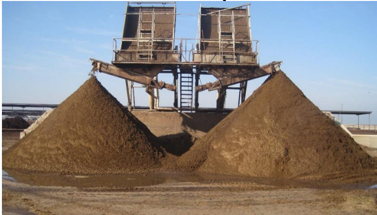
Figure 5: ABEC #3 Manure Solids Screen Separators and Resulting Fiber Stacks
